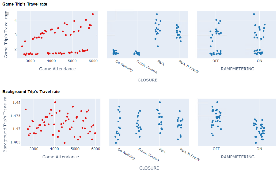
Figure 32: Scatter plots of travel rates with respect to uncertainties and policy levers in TransDNA experiments
